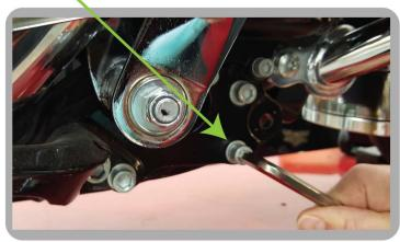
5. Put Ciro right mount in place and reinstall floorboard pivot pin and nut. Torque to 60-80 in-lbs.
