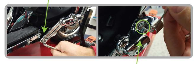
10. If using Ciro Click Peg Mounts, install 4-40 x 3/8" BSHCS and tab spring with a 1/16" hex wrench. Install Ciro footpeg with a D spring and 3/8"-24 x 1-1/8" SHCS.
