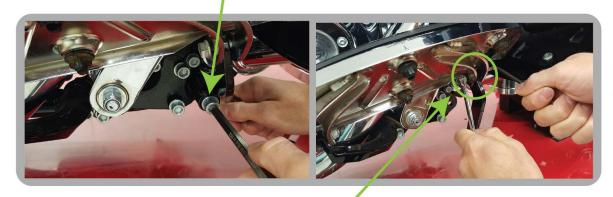
3. Using a 3/16" hex wrench and 7/16" box wrench, remove floorboard pivot pin. Remove floorboard bracket. Set aside pin and nut for reuse.
