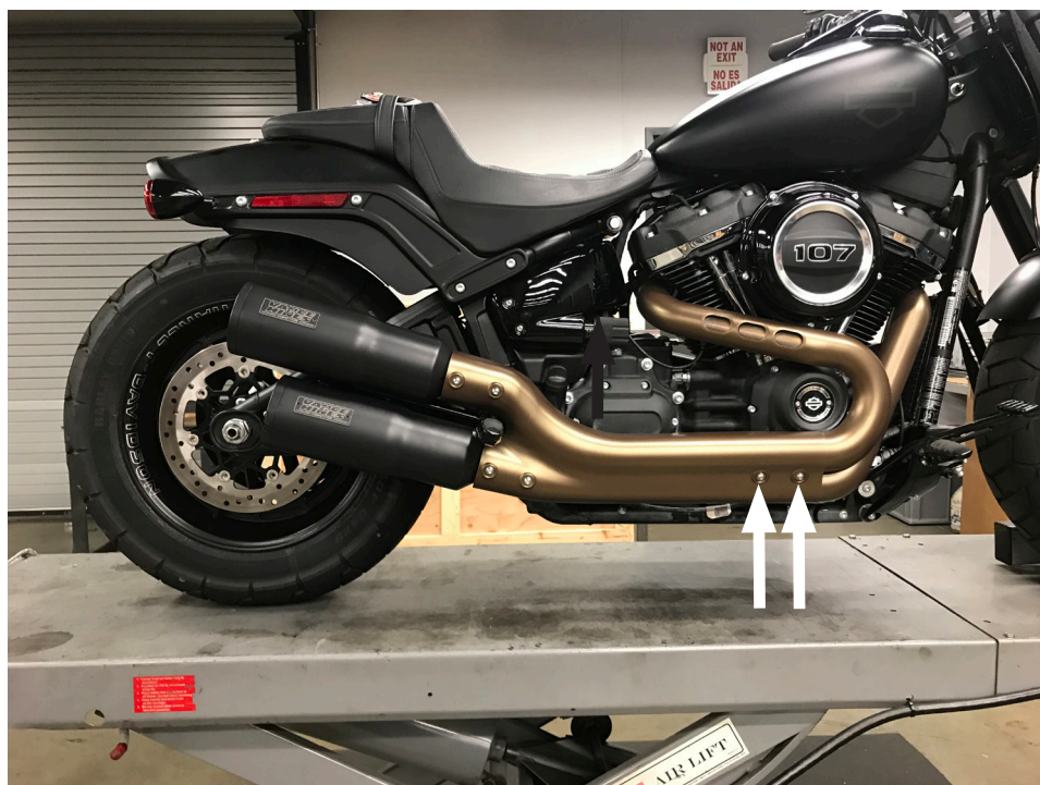
Install two forward fasteners first attaching heat shield to header.
