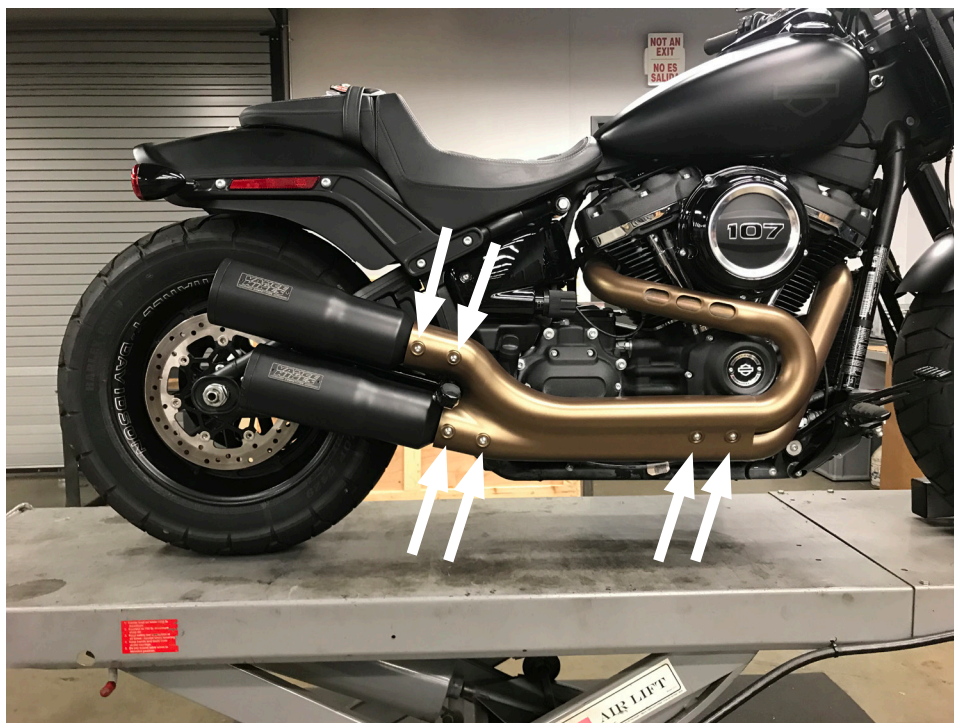
Remove six fasteners attaching head shield to header and mufflers
