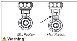
The adjustable end eye/bracket must not be threaded out more than that the groove is fully visible beneath the lock nut. This is maximum length. After adjusting, make sure that the lock nut is tightened (30Nm).
