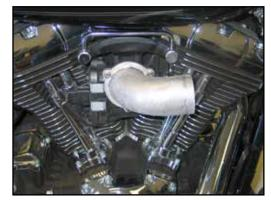
3. Loosen the three air filter retaining bolts shown.
