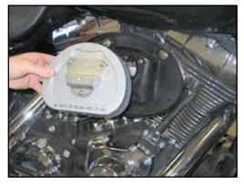
4. Remove the air filter from the vehicle and disconnect the crankcase breather tubes.
