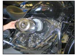
2. Remove the air filter cover bolt and air filter cover as shown.
