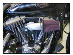
10. Install the provided K&N<sup>®</sup> air filter and secure with the provided hose clamp. A black hose clamp is being supplied with kit. This clamp is intended to clamp the filter to the intake tube. **NOTE: Drycharger<sup>®</sup> air filter wrap; Part # RC3680DK is available to purchase separately.**
