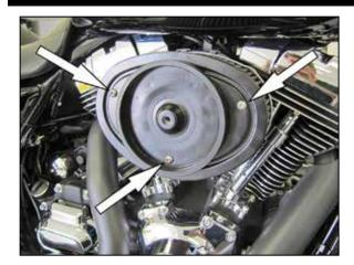
8. Install the  $K\&N^{\scriptsize @}$  air filter onto the back plate and secure with the provided hardware.
