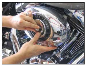
10. Install the bonnet onto the  $K\&N^{\otimes}$  air filter and secure with the factory bolt.
