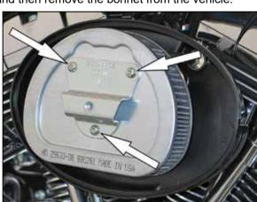
3. Remove the three bolts that secure the air filter and then remove the air filter and crank case breather tubes.
