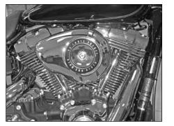
13. Remove the rubber gasket from the factory cover and then secure the cover to the filter assembly as shown.
