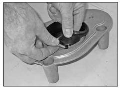
7. Install the three backing plate mounting bolts through the velocity stack.
