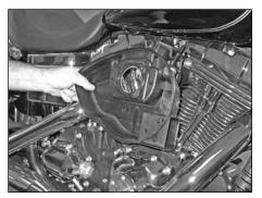
5. Remove the stock air filter base and gasket from the vehicle.
