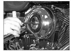
2. Remove the air filter cover mounting bolt and then remove the cover from the vehicle.
