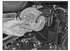
3. Remove the three air filter mounting bolts, unhook the two breather tubes from the breathers and then remove the air filter from the vehicle as
